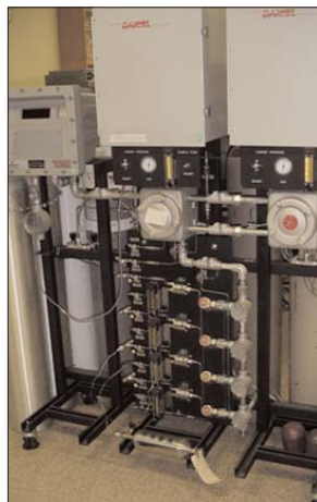
The BLM uses gas chromatographs to analyze gas samples from throughout the United States and the world, as part of investigations of the occurrences of helium in natural gases of countries with free-market economies. Photo courtesy of BLM.
